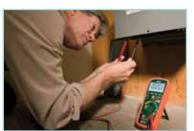
CAT IV application measuring voltage on a 480V 3-phase transformer
