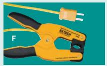
High Temperature Clamp probe (232°C) Conveniently fits 6.4 to 38mm pipes
