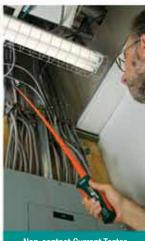
Wireless Circuit Detector for mid-run wires
