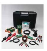
Datalogger and accessories are conveniently packaged in a protective hard carrying case
