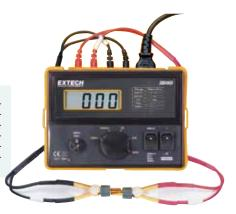
Complete with 4-wire cables with Kelvin clip connectors and power cord
