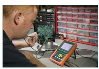
Dual trace testing or troubleshooting of printed circuit boards and electronic assemblies
