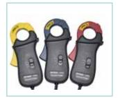
Optional 100A Current Clamp Probes (Model 382097) with 30mm jaw size
