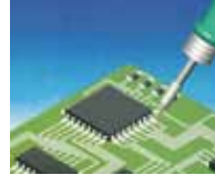
Soldering from 2 opposite angles
