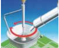
Desoldering IC component with hot air
