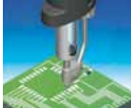
Cleaning pads with desoldering iron
