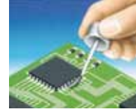
Fluxing IC pads and leads
