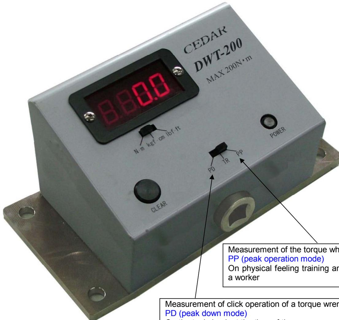
Measurement of the torque which actually started is here.
